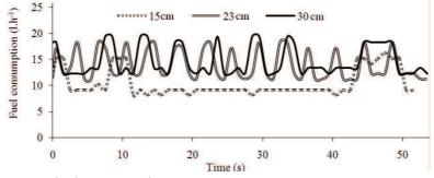
Fig. 3. Instantaneous fuel consumption by tractor engine.
